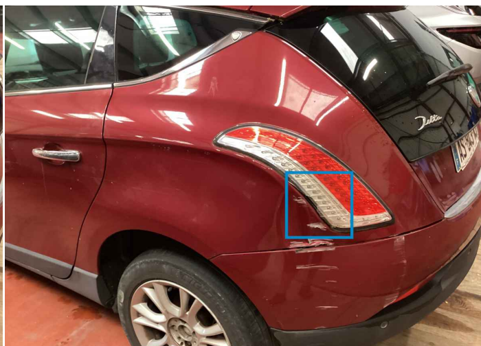
36. Fender / Back Left Bodywork / Breakage -
