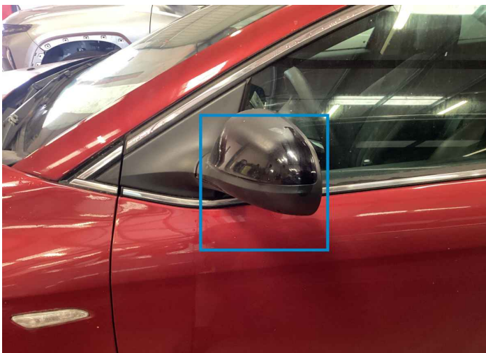
28. Mirror / Front Left Paint / Scratch / Scuff -
