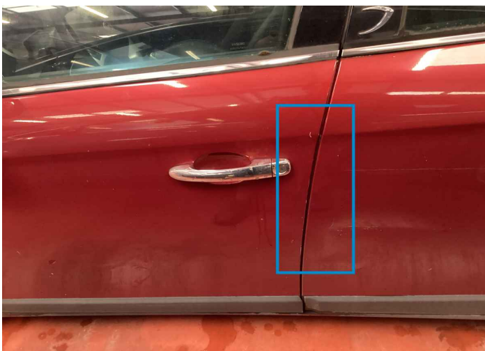
30. Door / Front Left Paint / Scratch / Line -
