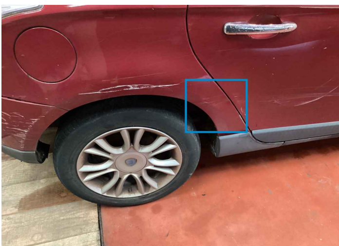
46. Fender / Back Right Bodywork / Dent / Deformation -
