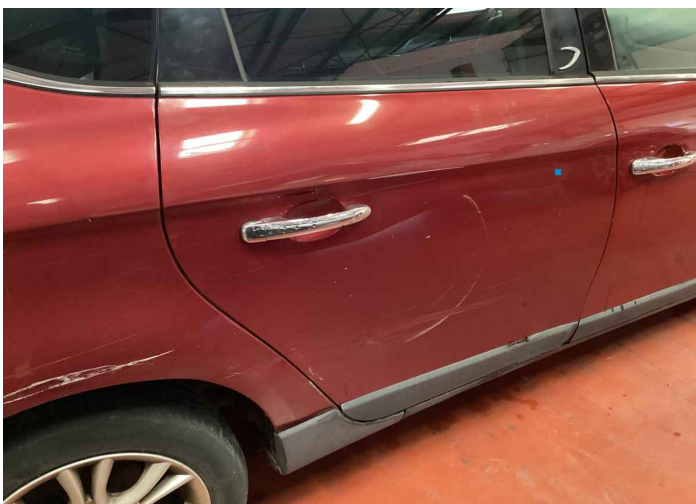
44. Door / Back Right Bodywork / Dent / Deformation -
