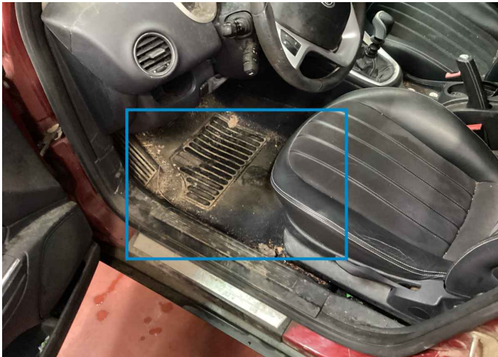
3. Floor Carpet Interior / Worn - out -
