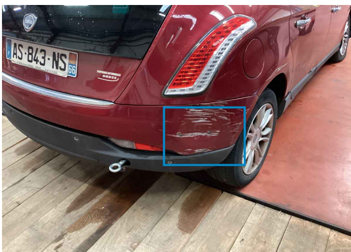
39. Corner Bumper / Back Right Bodywork / Dent / Deformation -
