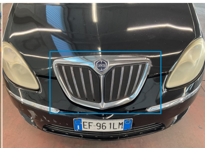
22. Grille / Front Bodywork / Breakage -
