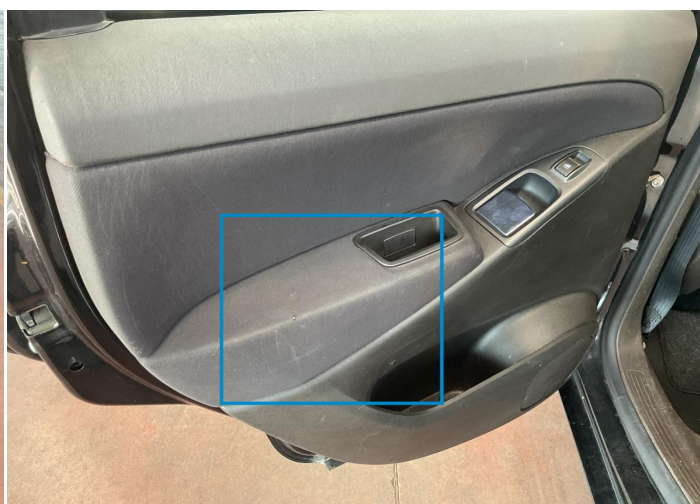
32. Panel Filling / Back Left Interior / Broken -
