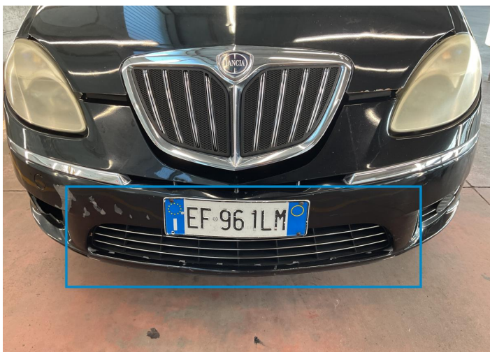
23. Shield Grid / Front Center Bodywork / Breakage -
