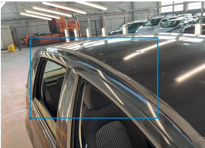
15. Pillar / Front Right Bodywork / Dent / Hail Area -
