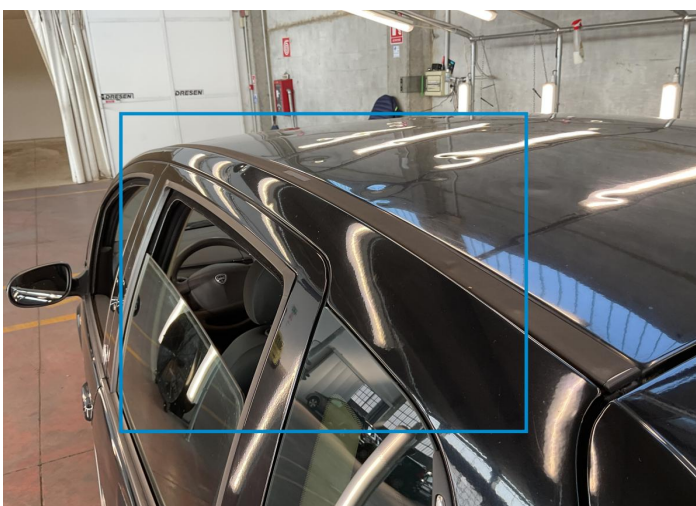
10. Pillar / Front Left Bodywork / Dent / Hail Area -
