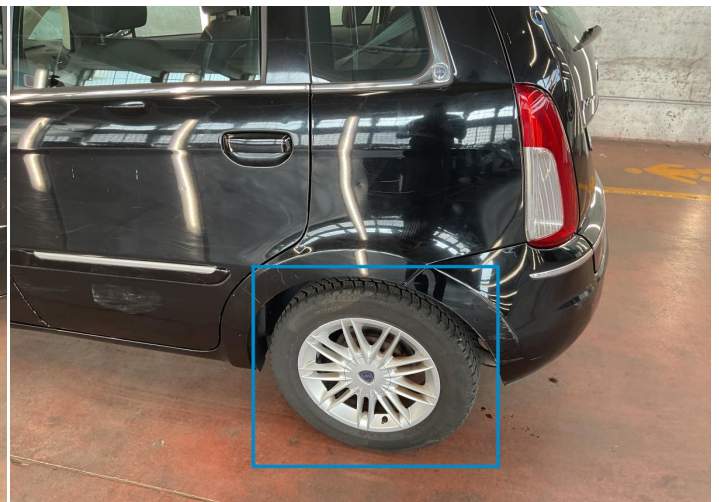
30. Rim / Back Left Out of Bodywork / Scratch -
