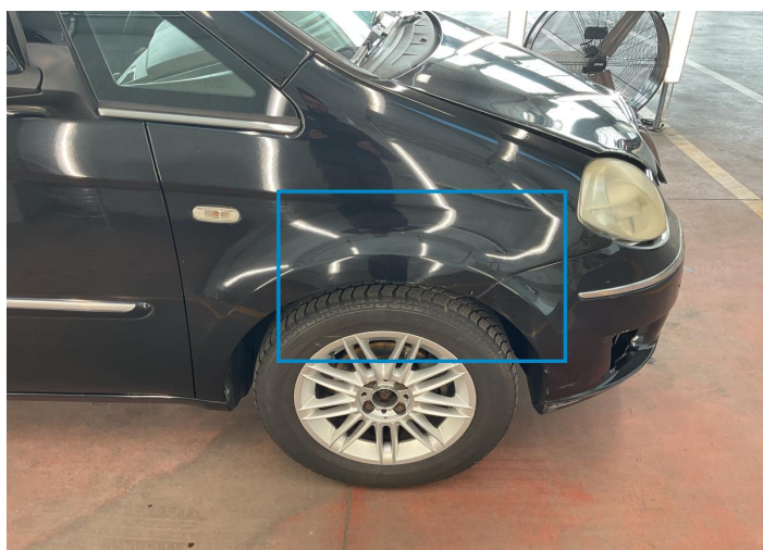
33. Fender / Front Right Bodywork / Dent -
