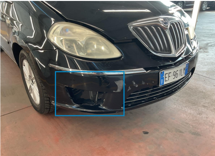
37. Shield Grid / Front Center Missing Part -
