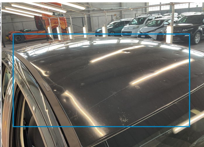
2. Roof Bodywork / Dent / Hail Area -
