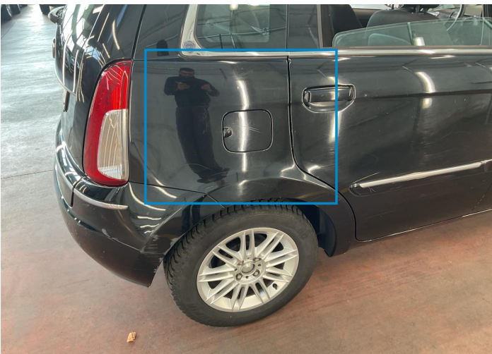
29. Fender / Back Right Bodywork / Dent -
