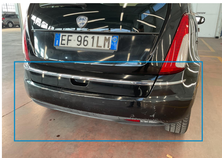
7. Bumper / Back Bodywork / Breakage -
