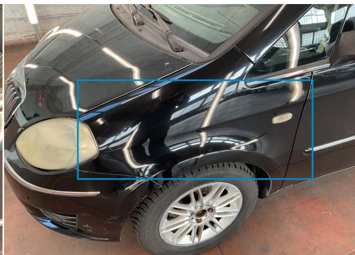
20. Fender / Front Left Bodywork / Dent / Hail Area -
