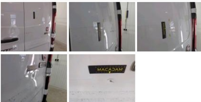
Supplementary brake light, Broken, Replace
