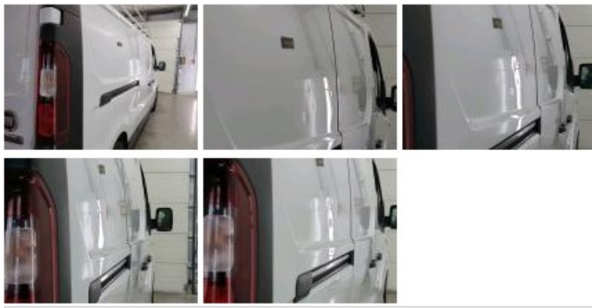
Sliding door R, Scratch(es), Repair and paint (complete)
