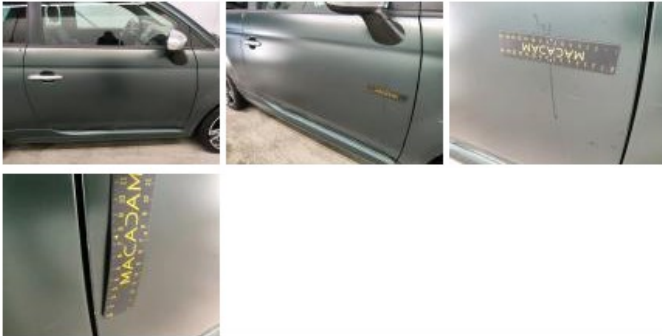
Wing FR, Scratch(es), Repair and paint (complete)
