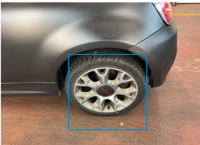
8. Rim / Back Left Out of Bodywork / Scratch -
