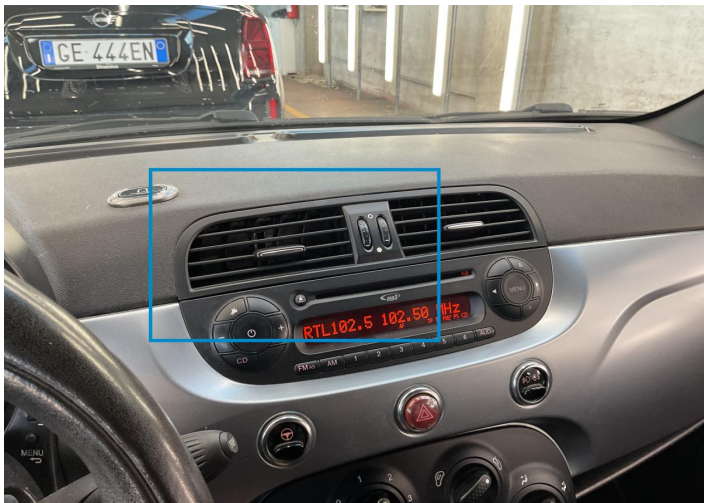
1. Aeration Grid / Front Center Interior / Broken -
