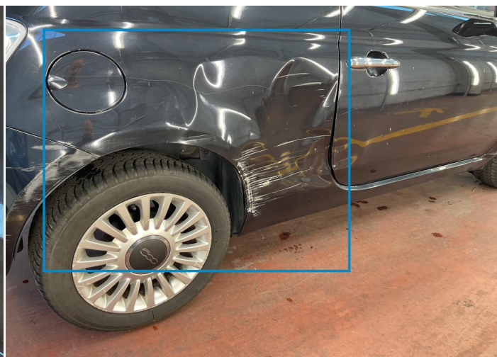
20. Fender / Back Right Bodywork / Dent -
