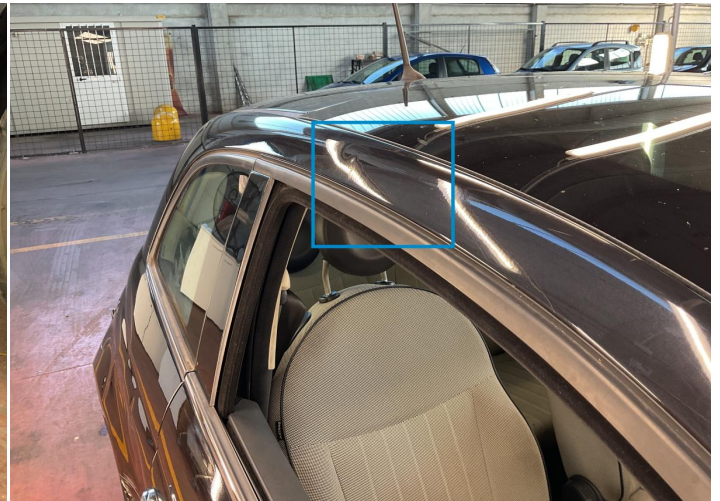
26. Pillar / Front Right Bodywork / Dent -
