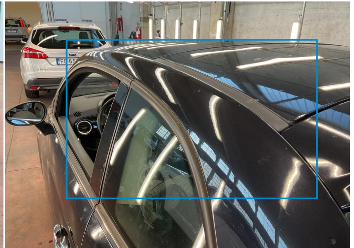
16. Pillar / Front Left Bodywork / Dent / Hail Area -
