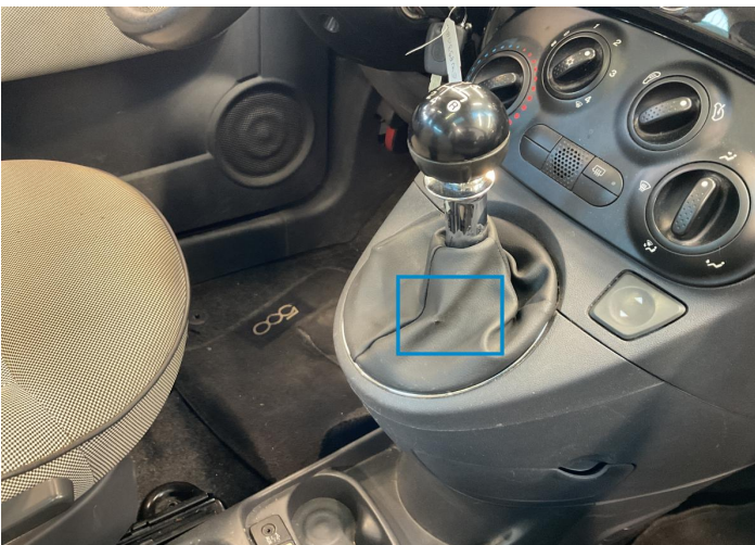
29. Gear Knob Interior / Ripped -
