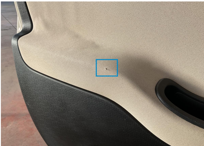
4. Panel Filling / Front Left Interior / Broken -
