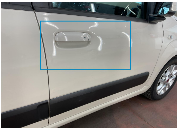
28. Door / Front Right Bodywork / Dent -
