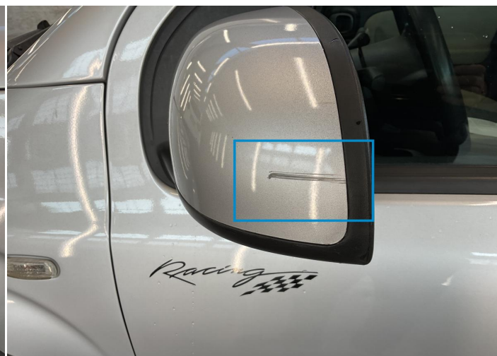
12. Mirror Shell / Front Left Paint / Scratch / Line -
