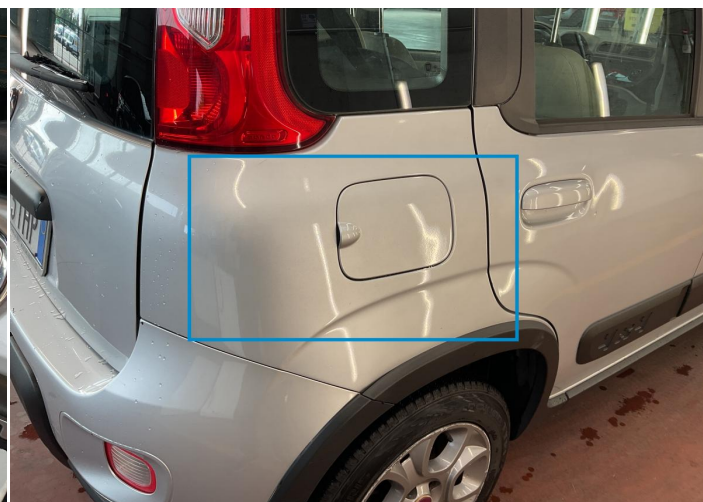
20. Fender / Back Right Bodywork / Poor Previous Repair -
