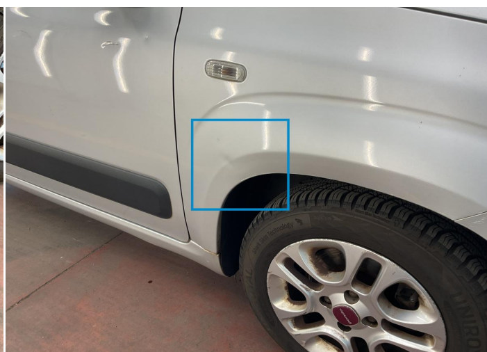
34. Fender / Front Right Bodywork / Dent -
