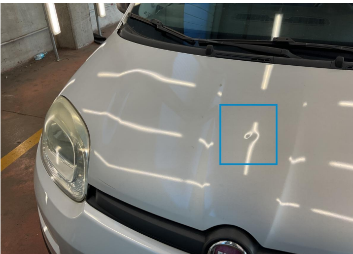
11. Hood Bodywork / Dent -
