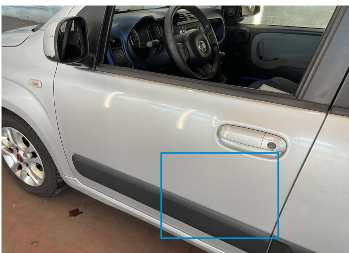
18. Door / Front Left Paint / Scratch / Line -
