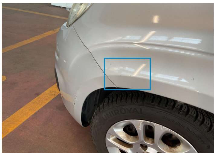
15. Fender / Front Left Bodywork / Dent -
