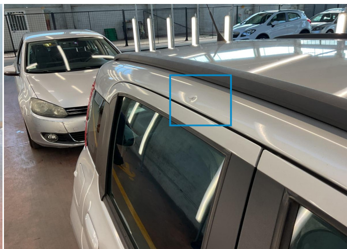
36. Pillar / Front Right Bodywork / Dent -
