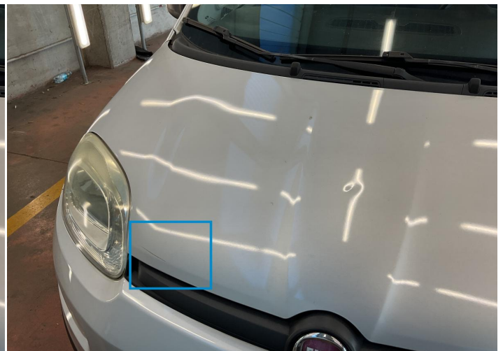
12. Hood Bodywork / Dent -
