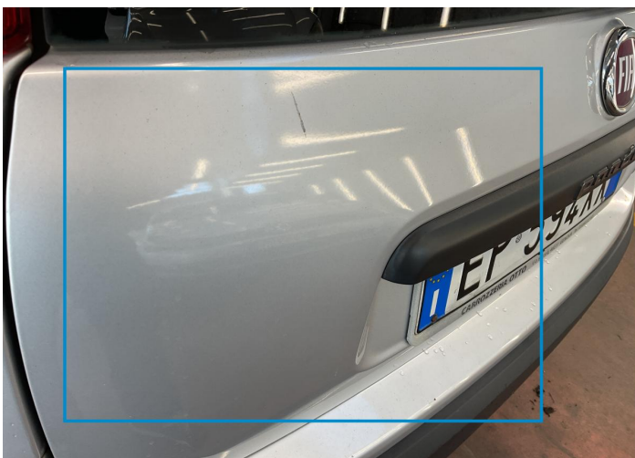
26. Tailgate Bodywork / Poor Previous Repair -
