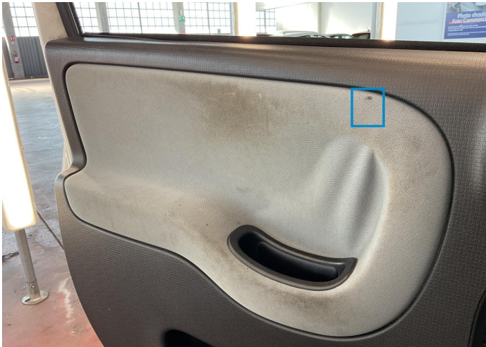
3. Panel Filling / Front Left Interior / Burn -
