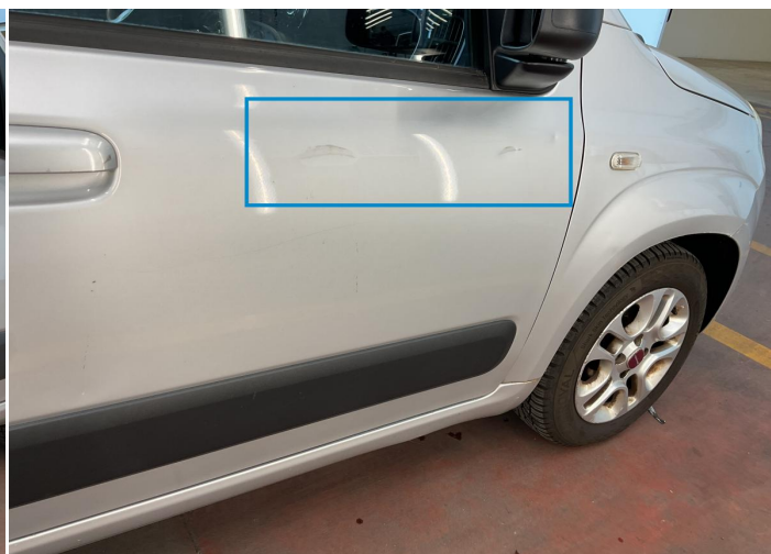
32. Door / Front Right Bodywork / Dent -
