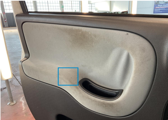
2. Panel Filling / Front Left Interior / Burn -
