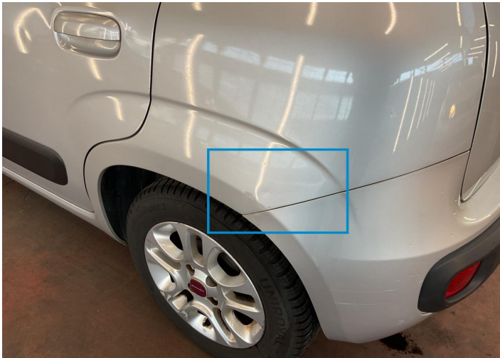
21. Fender / Back Left Bodywork / Dent -
