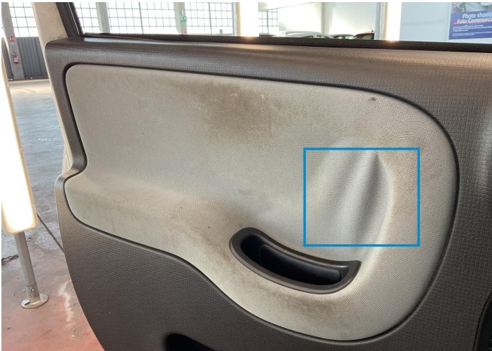
4. Panel Filling / Front Left Interior / Broken -
