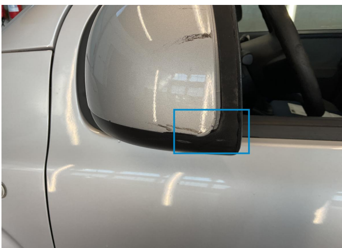
16. Mirror Shell / Front Left Bodywork / Breakage -
