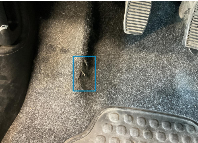
9. Floor Carpet Interior / Broken -
