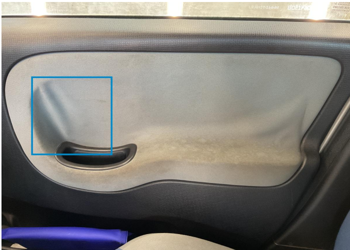
5. Panel Filling / Front Right Interior / Broken -
