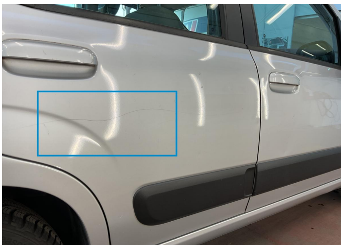
31. Door / Back Right Paint / Scratch / Line -
