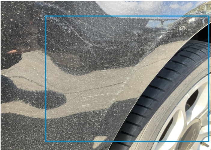
2. Fender / Back Left Paint / Scratch / Scuff -
