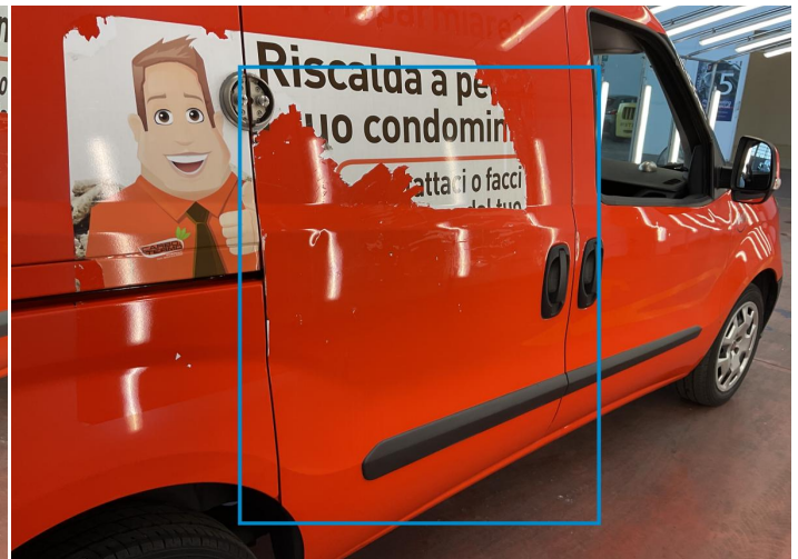
22. Door / Back Right Bodywork / Dent -
