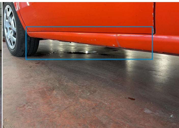
15. Rocker Panel / Center Left Bodywork / Dent -
