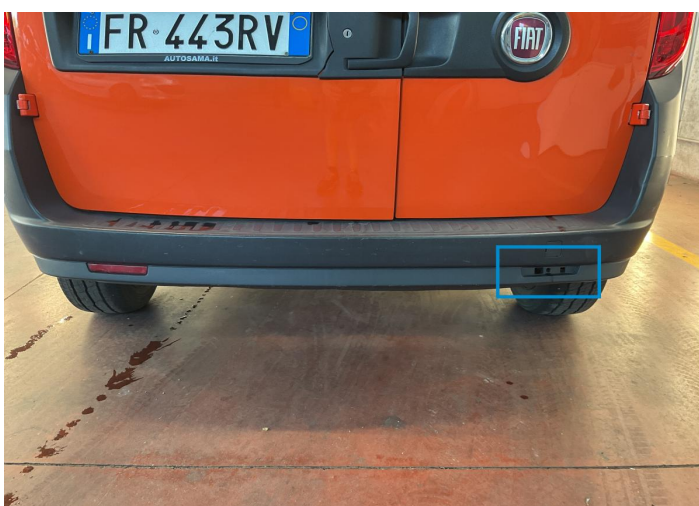
16. Reflector / Back Right Missing Part -
