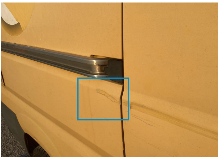
11. Side Panel / Back Right Bodywork / Dent / Deformation -
