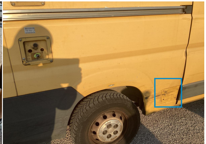
8. Side Panel / Back Right Missing Part -
