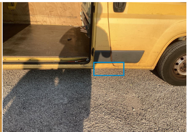
12. Rocker Panel / Center Right Bodywork / Dent / Deformation -
