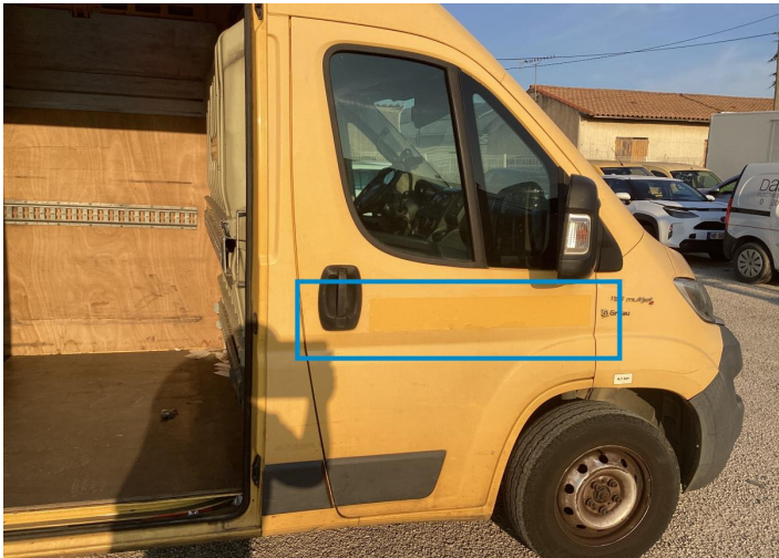
13. Door / Front Right Bodywork / Dent / Deformation -
