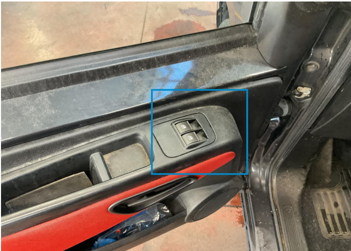
34. Window Switch / Front Left Interior / Dysfunctional - 0.00
