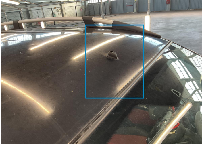
36. Antenna Rod Missing Part - 0.00
