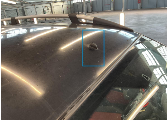
35. Antenna Base Bodywork / Breakage - 0.00
