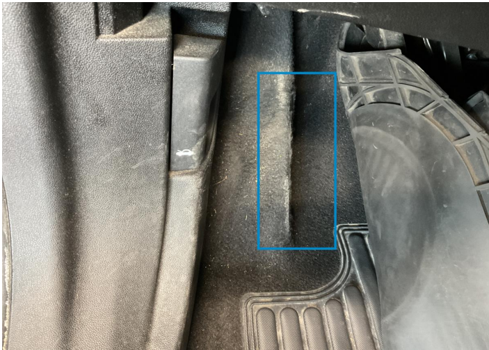
3. Floor Carpet Interior / Ripped -
