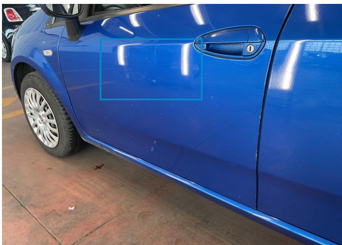
11. Door / Front Left Bodywork / Dent -
