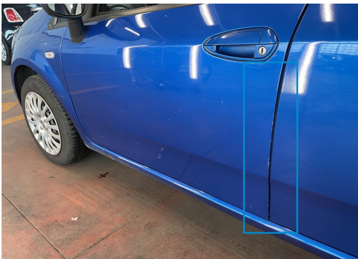
10. Door / Front Left Paint / Scratch / Line -
