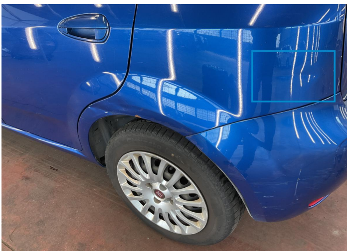
14. Fender / Back Left Bodywork / Dent -
