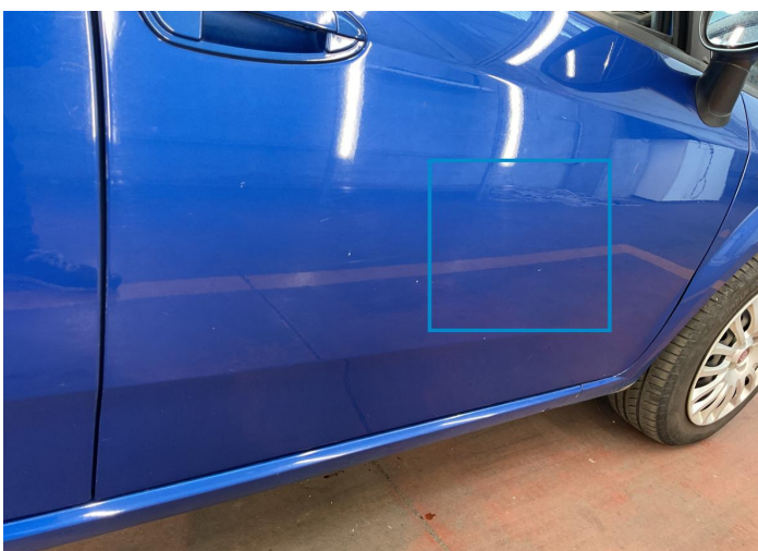
22. Door / Front Right Paint / Scratch / Line -
