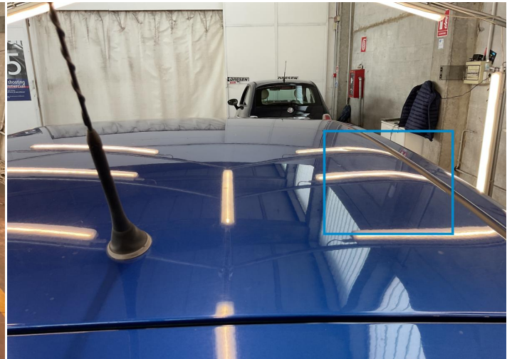
26. Roof Bodywork / Dent -
