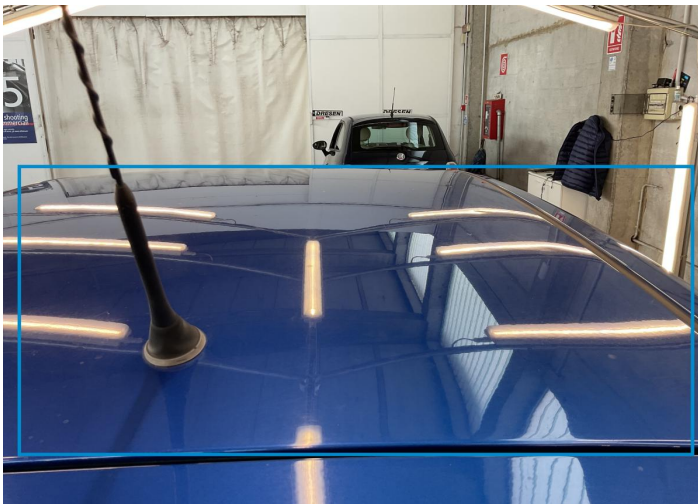
27. Roof Bodywork / Dent / Hail Area -
