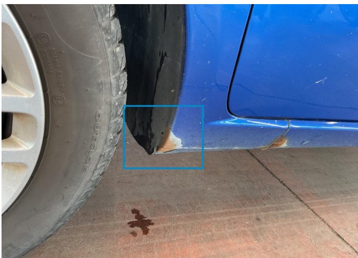
8. Fender / Front Left Bodywork / Dent -
