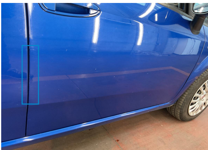
21. Door / Front Right Paint / Scratch / Line -
