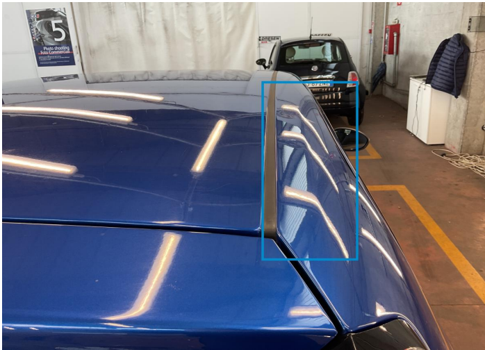
25. Pillar / Front Right Bodywork / Dent -
