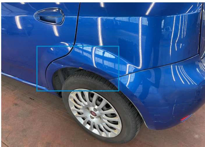
13. Fender / Back Left Bodywork / Dent -
