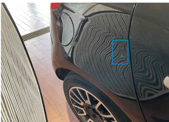
11. Fender / Back Right Bodywork / Dent / Dent -
