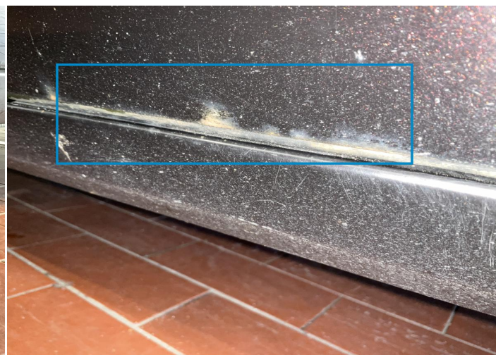
6. Door / Front Left Paint / Scratch / Line -
