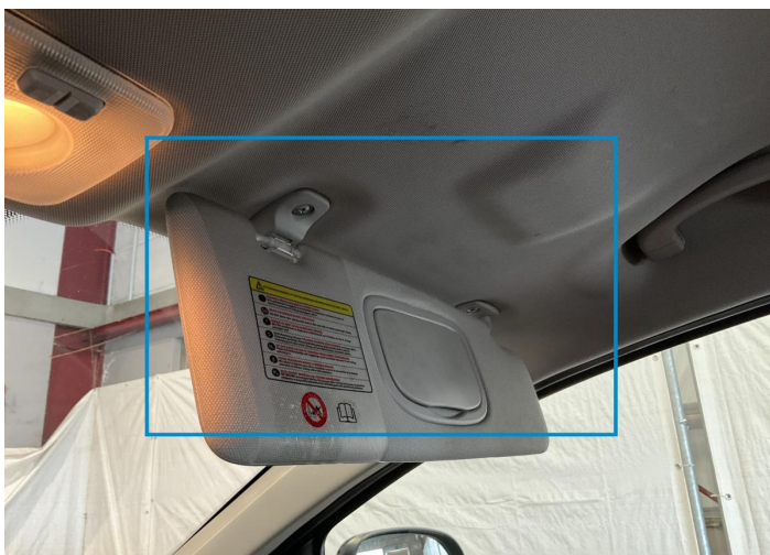
7. Sun Visor / Front Right Interior / Loose -
