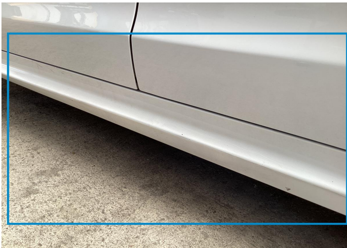
13. Rocker Panel / Center Left Paint / Scratch / Line -
