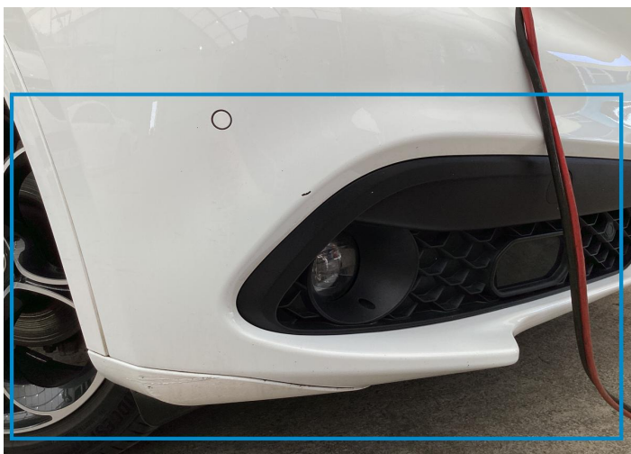
5. Corner Bumper / Front Right Paint / Scratch / Line -
