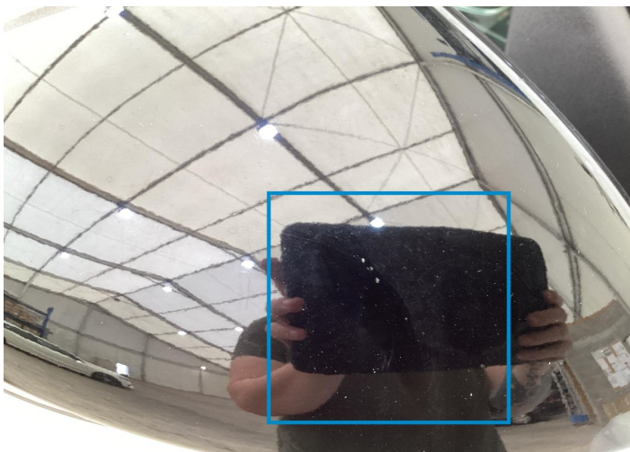
3. Mirror Shell / Front Right Paint / Chipping -
