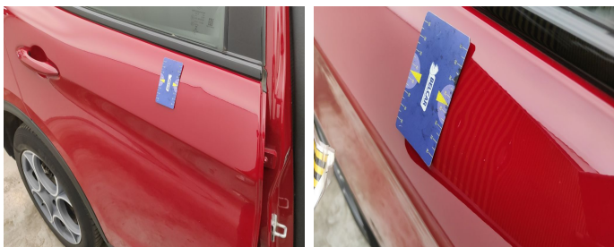
Door Rear Right // Repair & Painting-scratch + dent
