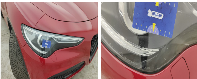
Light / Front Right / Replace-scratch
