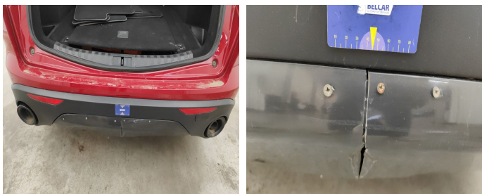
Bumper Rear / Spoiler / Replace-cracked
