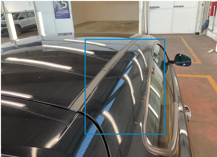
15. Pillar / Front Right Bodywork / Dent / Hail Area -
