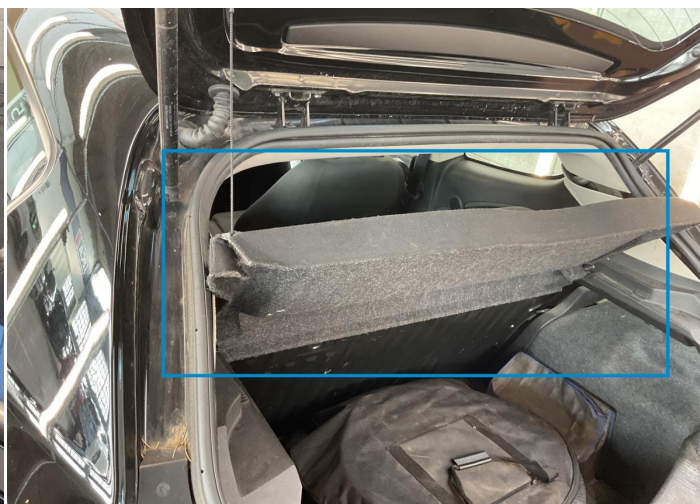
8. Luggage Space Cover / Back Interior / Broken -
