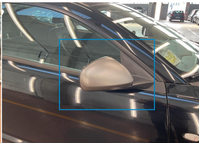
12. Mirror Shell / Front Right Paint / Scratch / Line -
