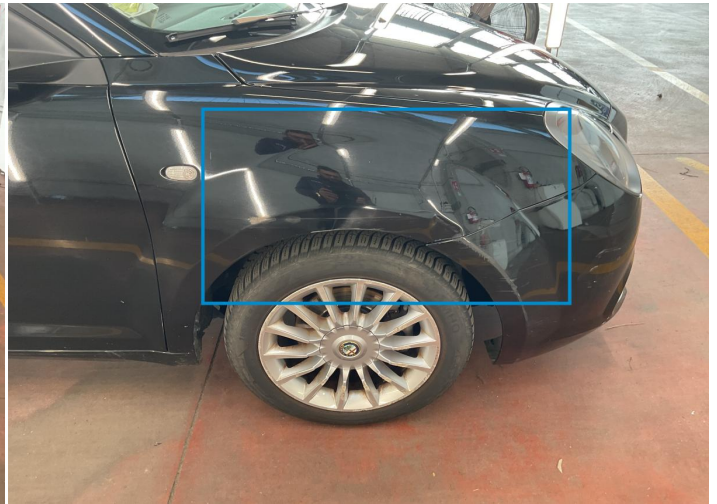
16. Fender / Front Right Bodywork / Dent -
