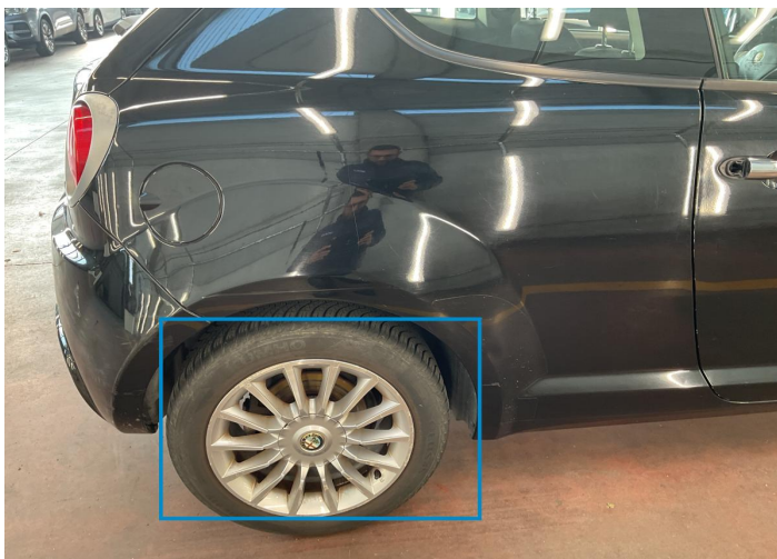
21. Rim / Back Right Out of Bodywork / Scratch -
