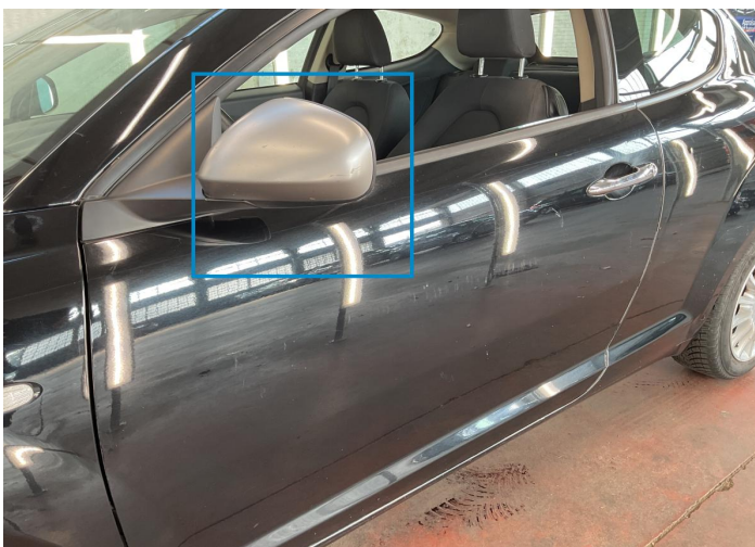
24. Mirror Shell / Front Left Paint / Scratch / Line -
