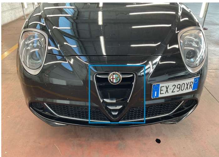
25. Grille / Front Bodywork / Breakage -
