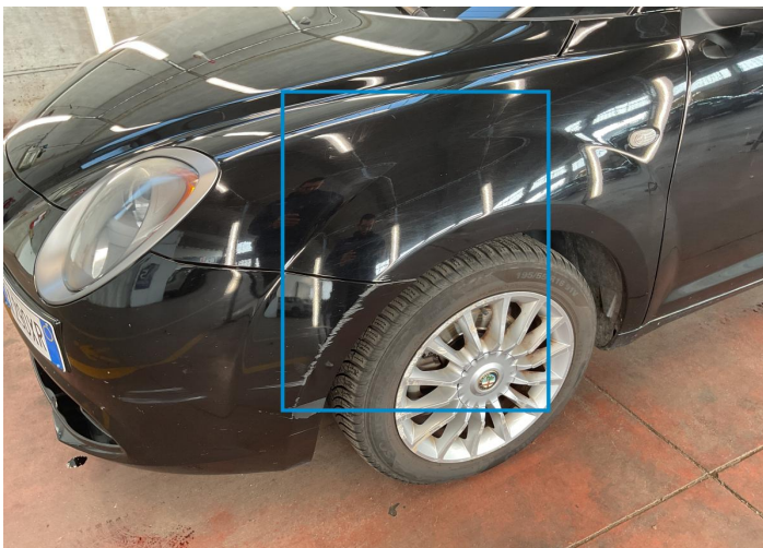
17. Fender / Front Left Bodywork / Dent -
