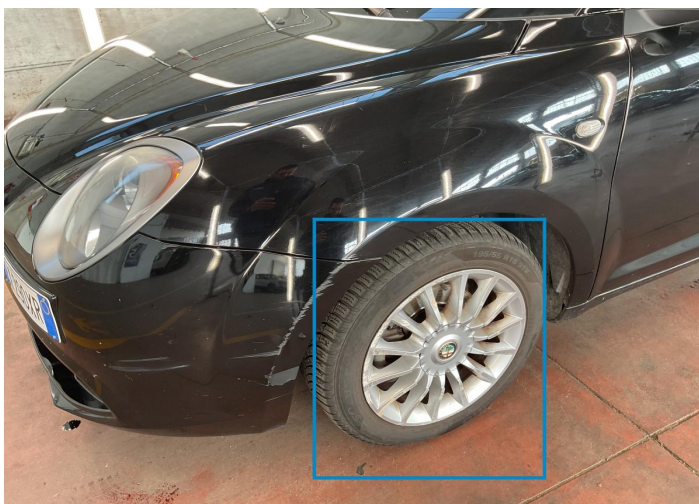
19. Rim / Front Left Out of Bodywork / Scratch -
