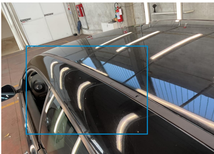
7. Pillar / Front Left Bodywork / Dent / Hail Area -
