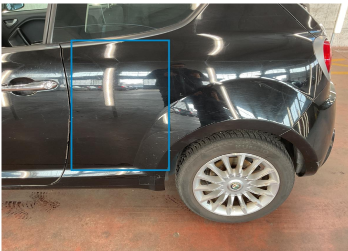
22. Fender / Back Left Bodywork / Dent -
