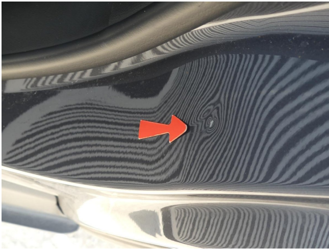
Tür hinten links - Einstieg-Kratzer-Smart Repair
