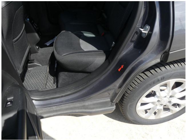
Tür hinten links - Einstieg-Kratzer-Smart Repair
