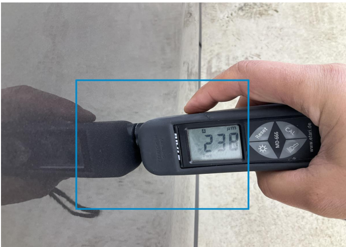
2. Door / Front Left Paint / Poor Previous Repair -
