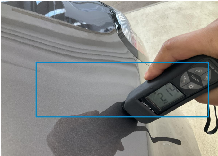
4. Side Panel / Back Left Paint / Poor Previous Repair -
