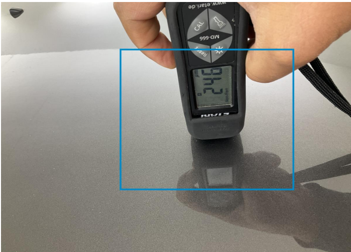
6. Hood Paint / Poor Previous Repair -
