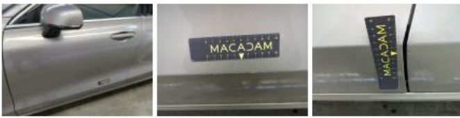
Door RL, Dent(s) and scratch(es), Repair and paint (complete)
