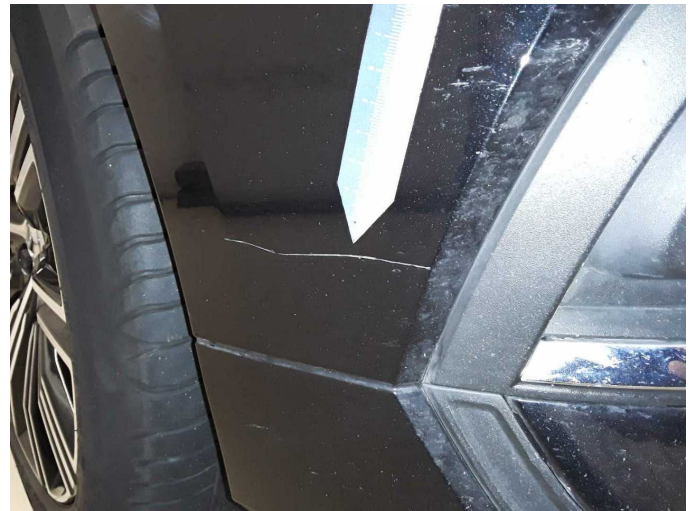
Damage 4: Front bumper: Front bumper - Scratch(es) - Repair and paint
