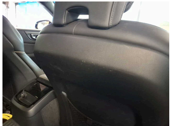
Damage 3: Seat - front: Backrest cover - right side (Schale hinten) - Scratch(es) - Smart repair
