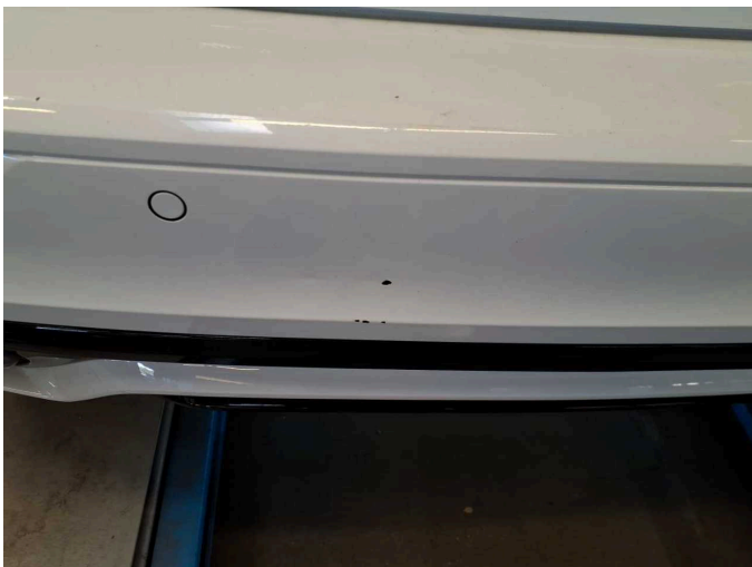
Damage 8: Rear bumper: Rear bumper - Scratch(es) - Paint
