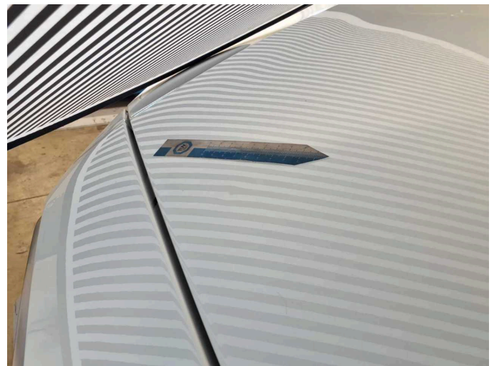
Damage 2: Bonnet: Bonnet - dent(s) - Smooth repair work
