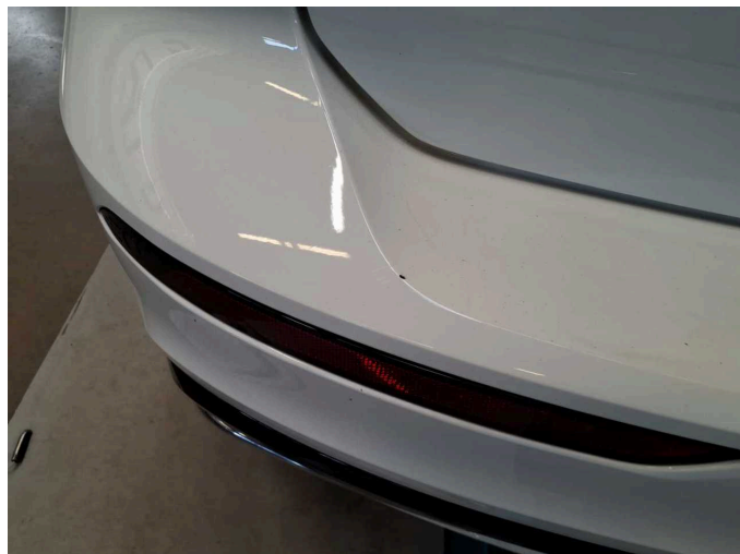
Damage 8: Rear bumper: Rear bumper - Scratch(es) - Paint
