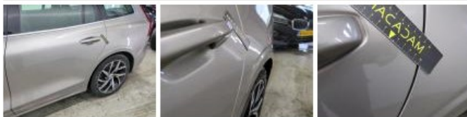
Door FL, Scratch(es), Repair and paint (complete)
