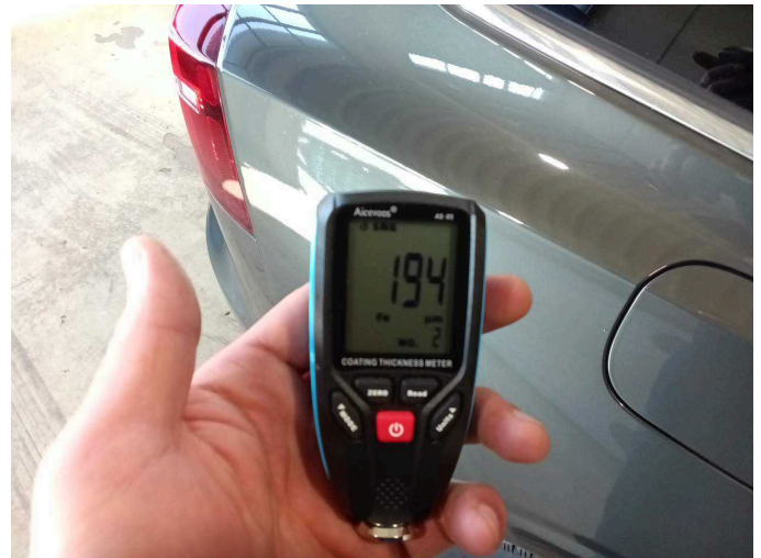
Side panel - rear right side: 194 µm
