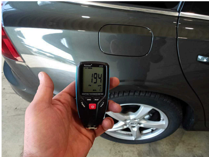
Side panel - rear right side: 194 µm
