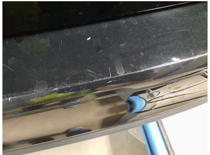
Damage 4: Rear bumper: Rear bumper - Scratched - Paint
