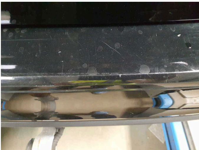
Damage 4: Rear bumper: Rear bumper - Scratched - Paint
