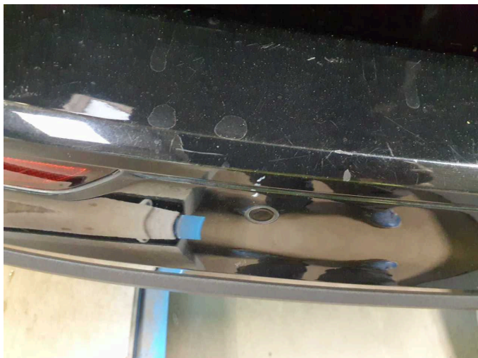
Damage 4: Rear bumper: Rear bumper - Scratched - Paint
