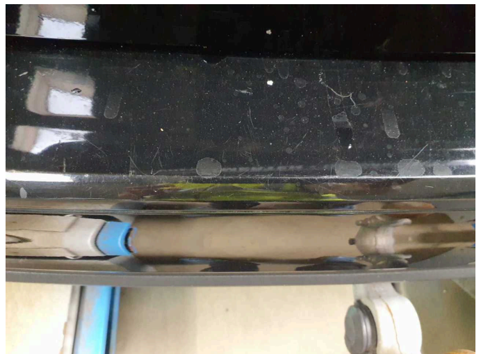
Damage 4: Rear bumper: Rear bumper - Scratched - Paint
