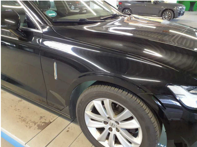
Damage 3: Mudguard - right side: Mudguard - right side - Scratched - Paint
