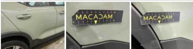
Wheel arch cover RR, Scratch(es), Replace
