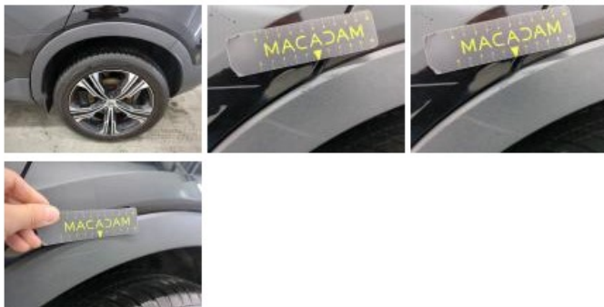
Bumper F, Scratch(es), Repair and paint (complete)
