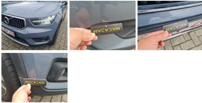
Bumper moulding F, Deformed / Strained, Replace
