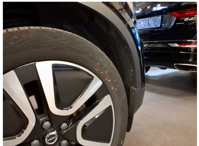
Damage 4: Wheel / tyres: Tyre - front right side - Porous / cracked - Replace
