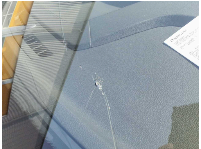
Damage 3: Vehicle glazing: Windscreen - Stone chips - repair according to calculation
