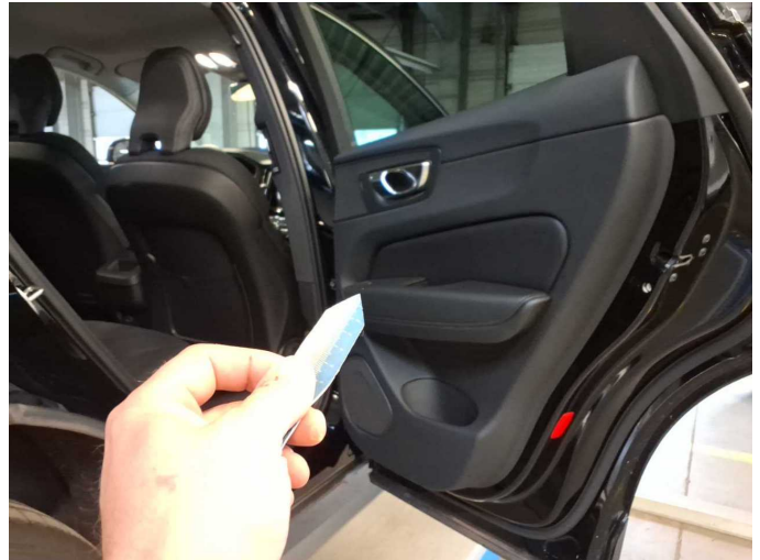
Damage 4: Trim / covers: Door trim - rear right side (Griff) - Broken / torn - Smart repair
