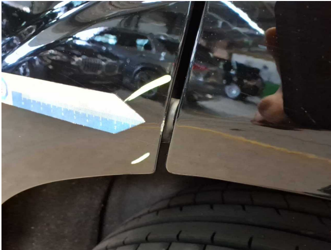
Wear and tear 2: Door - rear left side: Door edge - Scratch(es) - Smart repair
