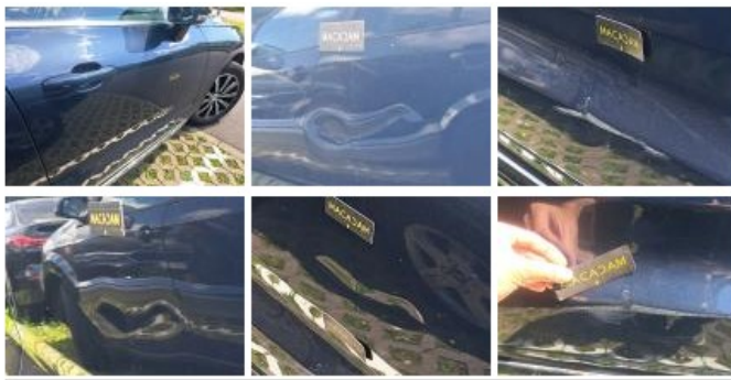
Door trim FR, Scratch(es), Repair and paint (complete)
