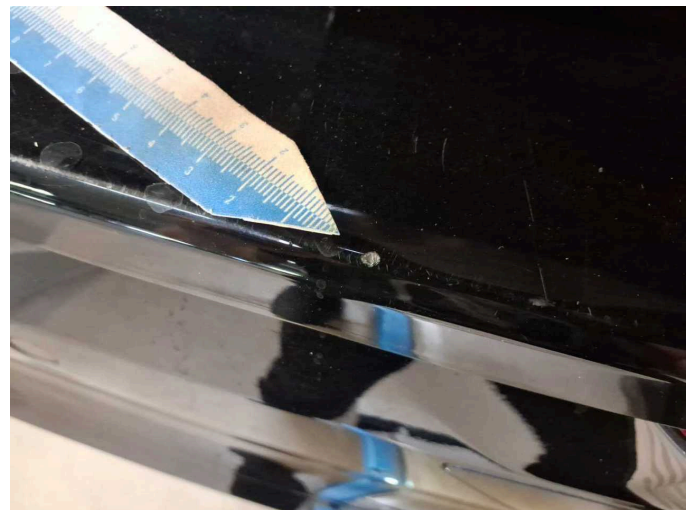
Damage 8: Rear bumper: Rear bumper - Scratch(es) - Paint
