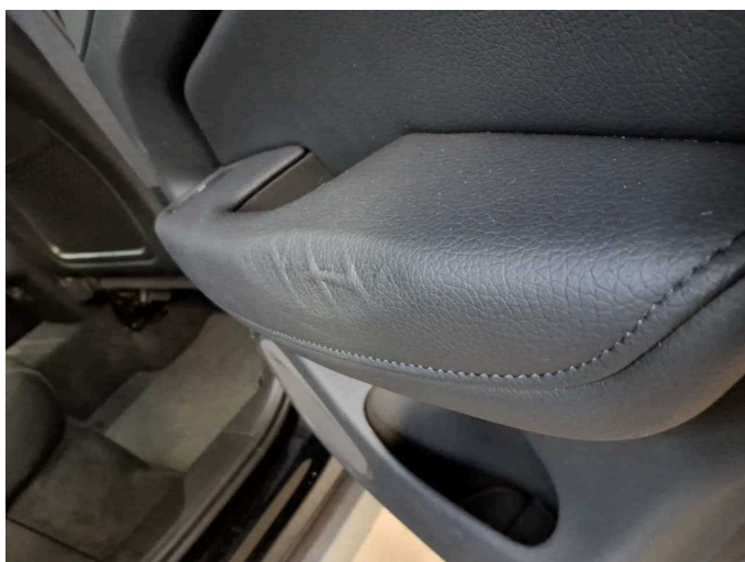
Damage 7: Trim / covers: Door trim - rear right side (Griff) - Deformed - Replace
