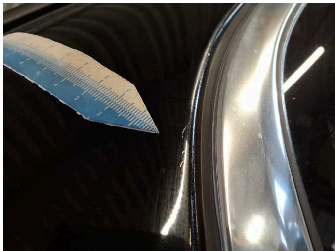
Damage 9: Side panel - rear right side: Side panel (Dellen, Kratzer. Übergang stumpf, schlecht vorbereitet) - Unprofessionally repaired - Repair and paint
