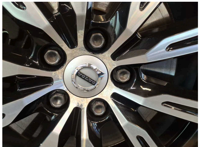
Damage 5: Wheel / tyres: Alloy rim - front left side - Paint defect - Loss in value
