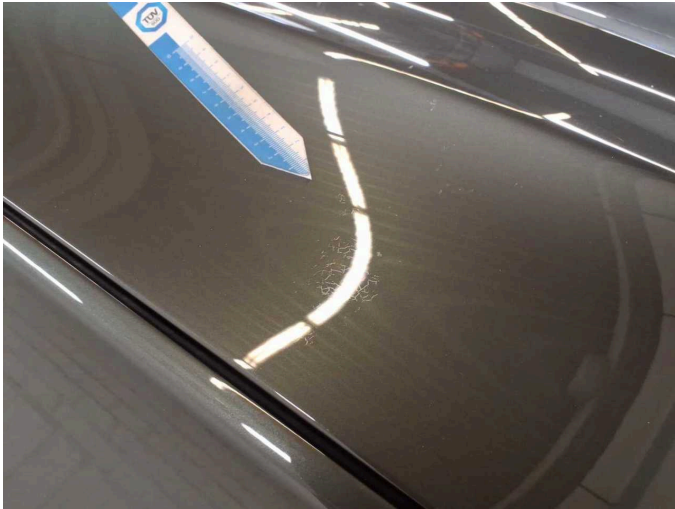
Damage 9: Bonnet: Bonnet - Paint defect - Paint
