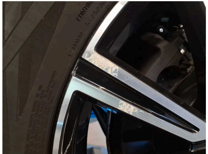
Damage 6: Wheel / tyres: Alloy rim - rear left side - Paint defect - Loss in value
