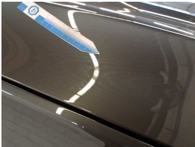
Damage 9: Bonnet: Bonnet - Paint defect - Paint
