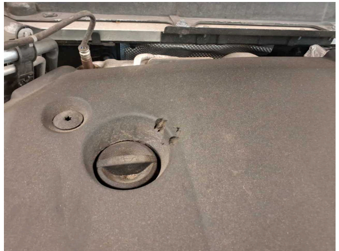
Damage 4: Engine: Engine cover - top / cover - Damage caused by marten / rodent - Replace
