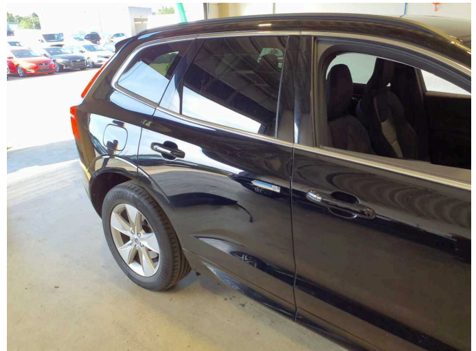
Wear and tear 4: Door - rear right side: Door - dent(s) - Smooth repair work
