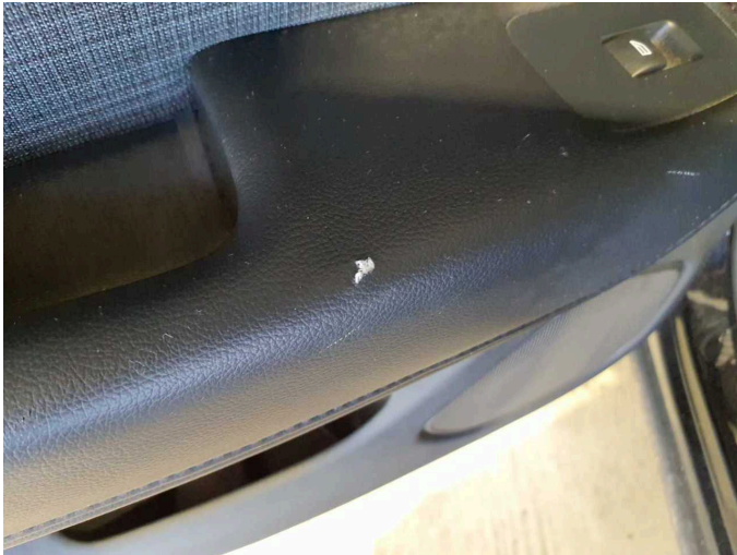
Damage 12: Trim / covers: Door trim - rear left side - Damaged - Loss in value
