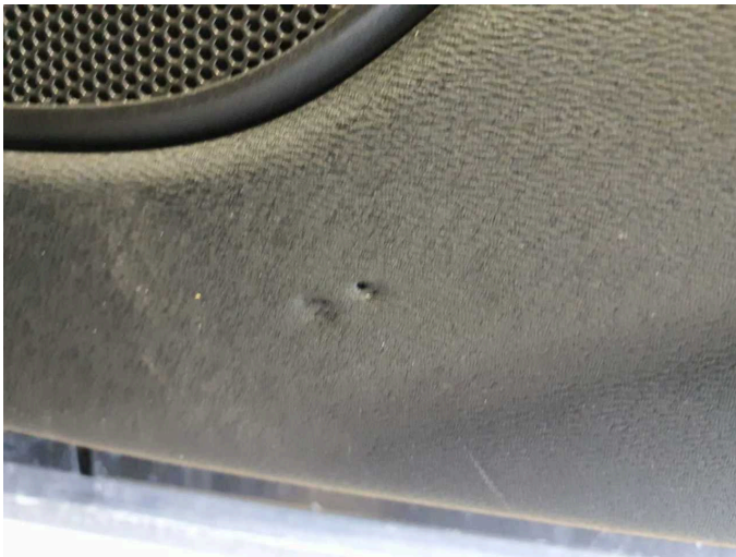
Damage 9: Trim / covers: Door trim - rear right side - dent(s) - Loss in value
