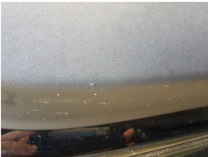
Damage 11: Trim / covers: Door trim - front left side - dent(s) - Loss in value
