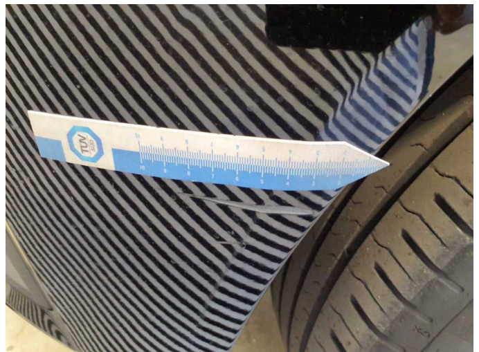
Damage 14: Front bumper: Front bumper - Scratch(es) - Paint
