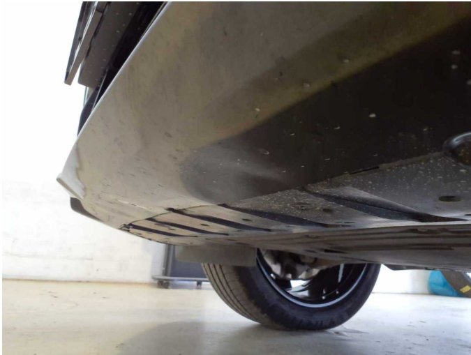
Damage 3: Front bumper: Spoiler - Deformed - Replace
