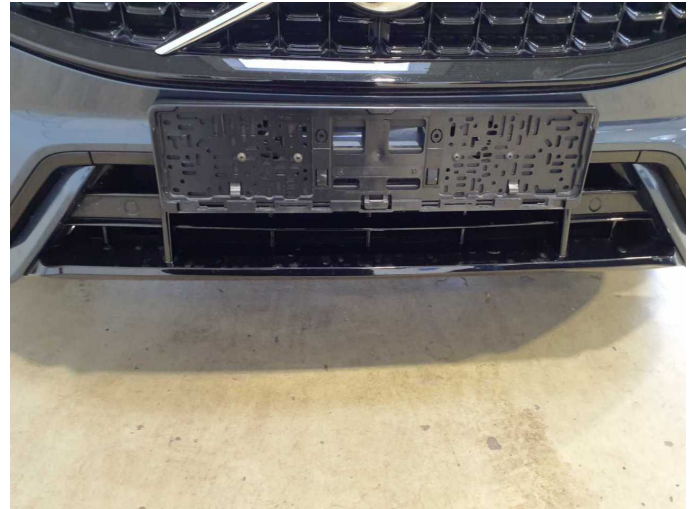
Damage 3: Front bumper: Spoiler - Deformed - Replace
