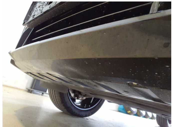
Damage 3: Front bumper: Spoiler - Deformed - Replace
