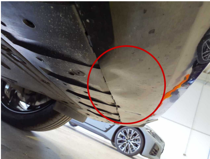
Damage 3: Front bumper: Spoiler - Deformed - Replace
