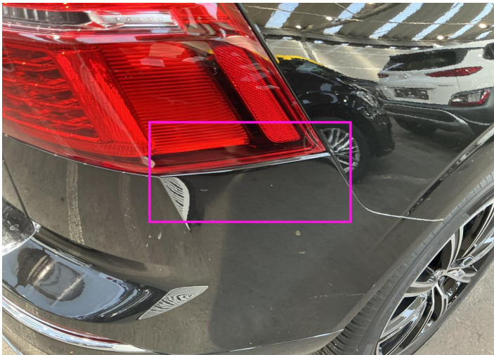
5. Bumper / Back Bodywork / Breakage -
