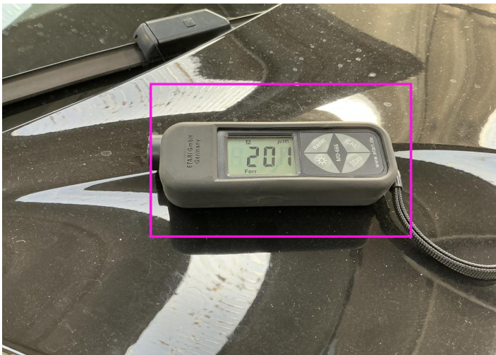
1. Door / Front Right Paint / Poor Previous Repair -
