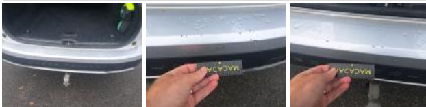
Bumper trim R, Scratch(es), Smart repair
