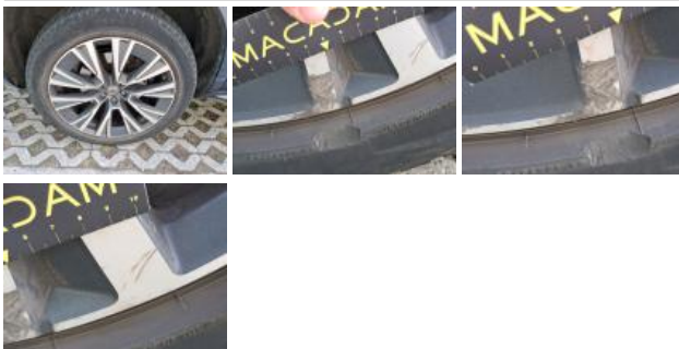
Tyre RR, Tear, Replace
