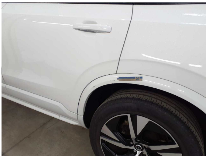
Damage 1: Side panel - rear left side: Wheel well extension - Scratch(es) - Smart repair
