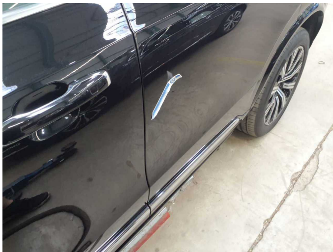
Damage 1: Door - rear left side: Door - Deformed - Repair and paint
