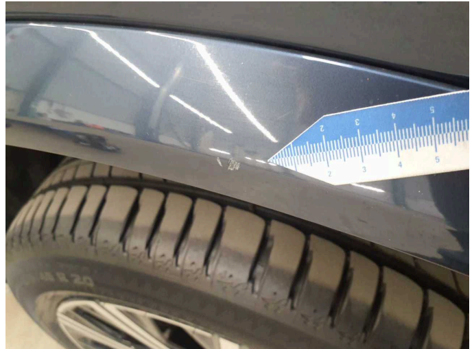
Damage 3: Side panel - rear left side: Wheel well extension - Scratched - Smart repair
