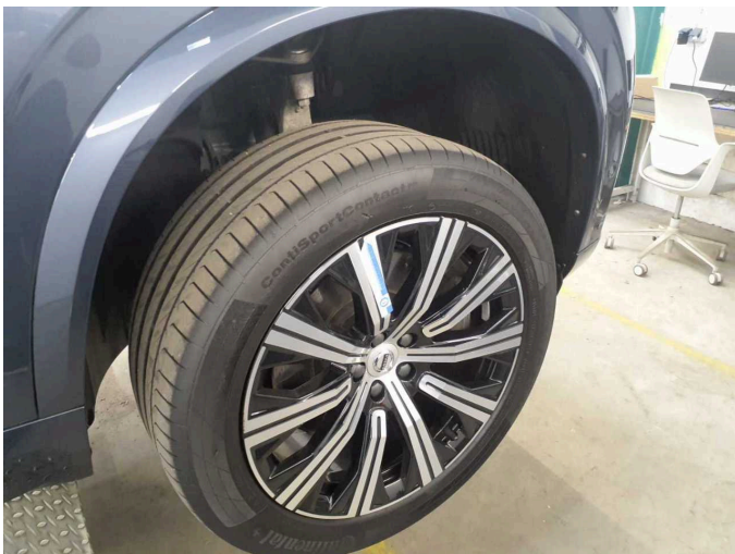
Damage 5: Wheel / tyres: Tyre - front right side (Flankenbeschädigung) - Damaged - Replace
