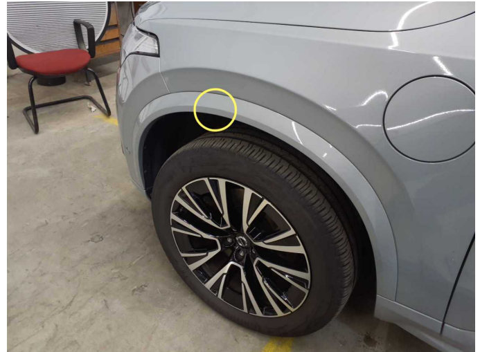
Damage 1: Mudguard - left side: Wheel well extension - Scratch(es) - Smart repair
