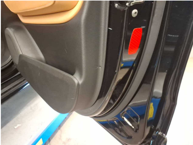
Damage 4: Trim / covers: Door trim - front right side - Scratch(es) - Smart repair
