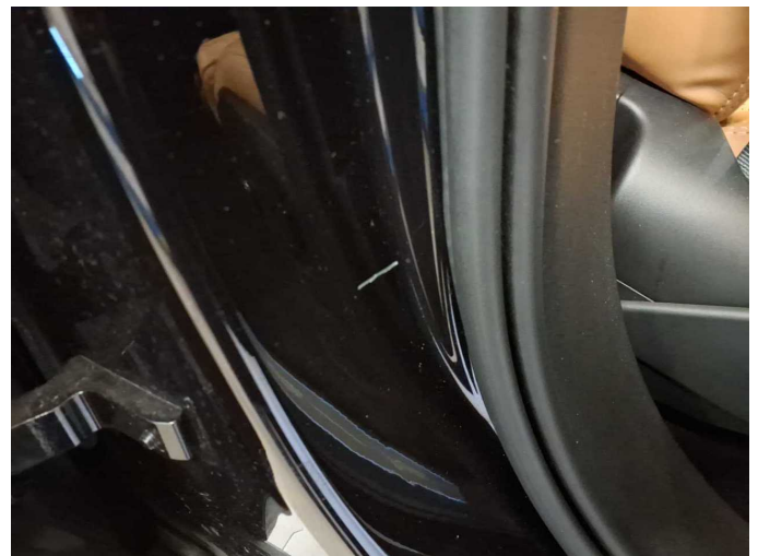
Damage 2: Body: B-pillar - right side - Scratch(es) - Smart repair
