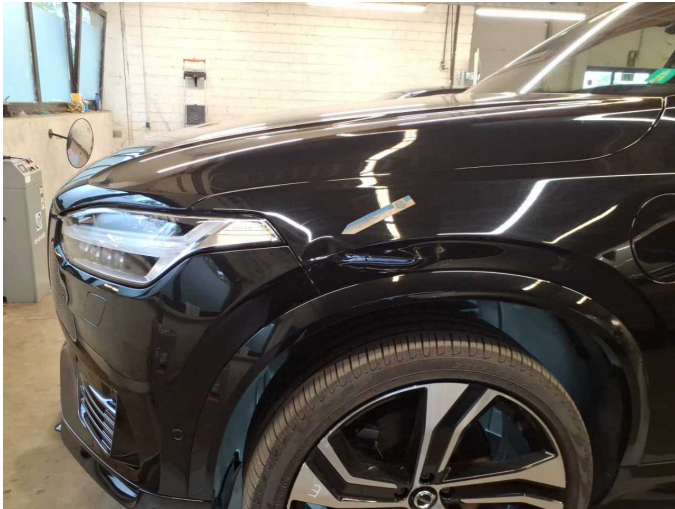
Damage 14: Mudguard - left side: Mudguard - left side - Dent / paintcoat damage - Replace
