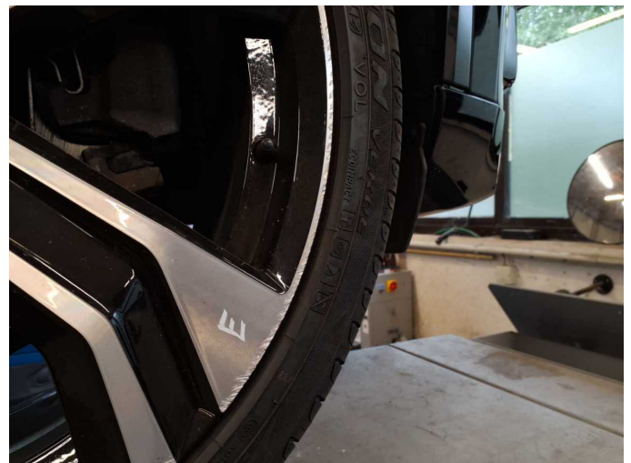
Damage 11: Wheel / tyres: Alloy rim - front right side - Scratched - Loss in value
