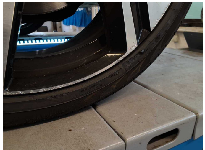
Damage 6: Wheel / tyres: Tyre - front right side (nicht fahrbereit) - Damaged - Replace
