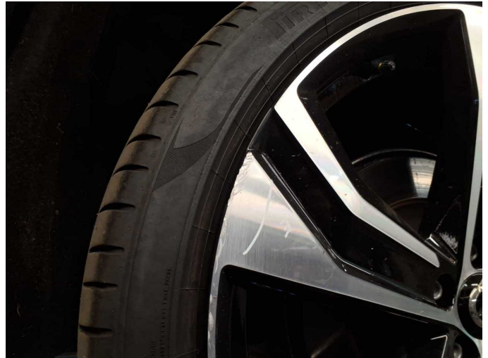
Damage 12: Wheel / tyres: Alloy rim - rear right side (Materialabtrag) - Scratched - Loss in value
