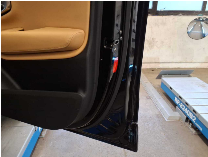
Damage 5: Door - front right side: Door (Innen) - dent(s) - Smooth repair work
