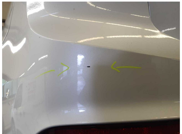
Damage 6: Rear bumper: Rear bumper - Scratch(es) - Paint
