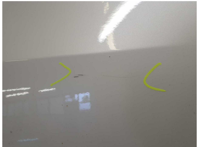
Damage 6: Rear bumper: Rear bumper - Scratch(es) - Paint
