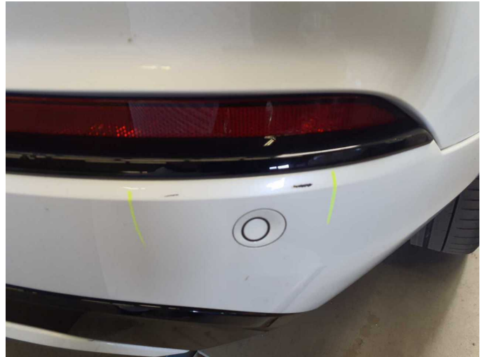
Damage 6: Rear bumper: Rear bumper - Scratch(es) - Paint
