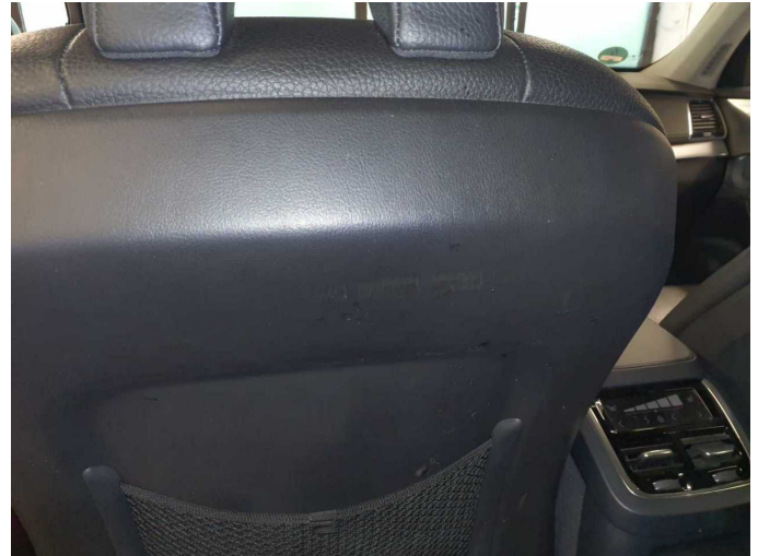
Damage 1: Seat - front: Backrest - left side (Reifenprofil) - Abrasion - Smart repair
