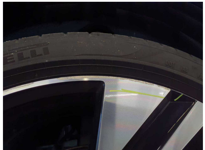
Damage 8: Wheel / tyres: Wheel rim - front left side (Materialabtrag) - Scratched - Replace
