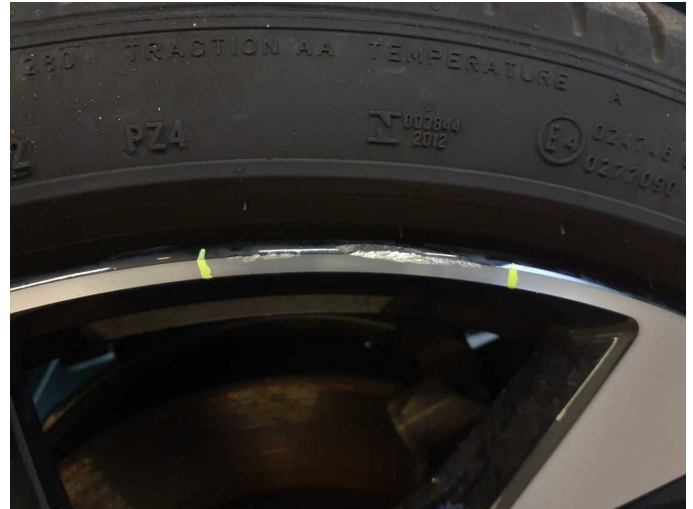
Damage 7: Wheel / tyres: Alloy rim - front right side (Materialabtrag) - Scratched - Replace
