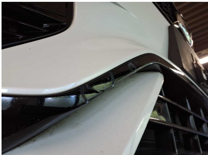
Damage 5: Front bumper: Front bumper (Zierleiste) - Deformed - Replace
