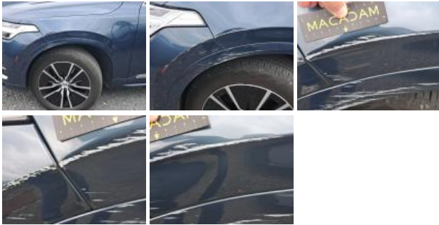
Wing trim FL, Scratch(es), Repair and paint (complete)
