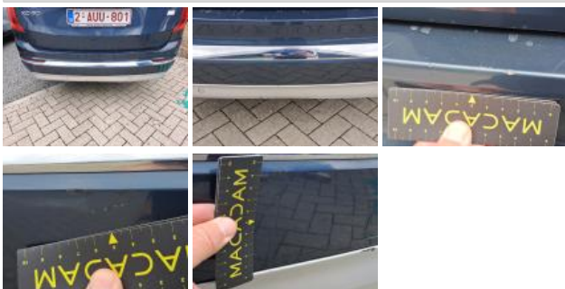
Bumper moulding R, Broken, Replace
