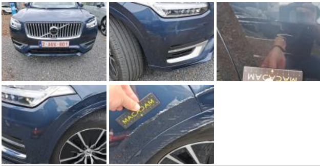
Wing FL, Dent(s) and scratch(es), Repair and paint (complete)
