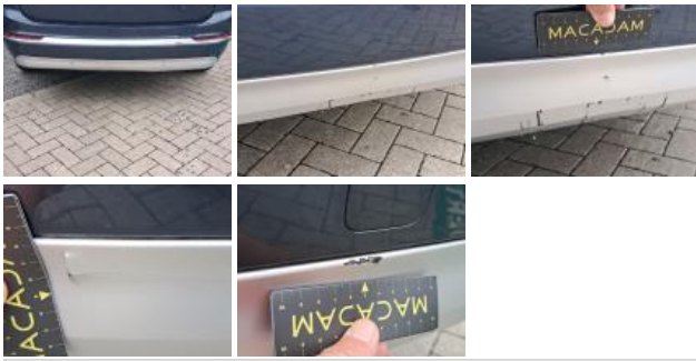
Tailgate / Boot, Dent(s), Paintless dent repair
