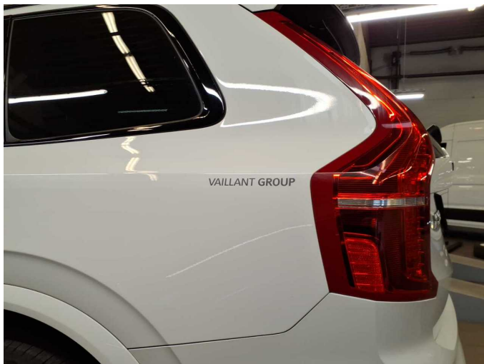
Damage 3: Side panel - rear left side: Side panel - Glued / labelled - De-glue / neutralise
