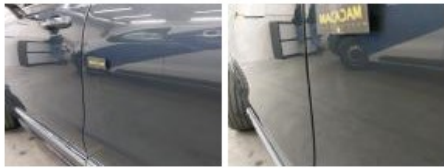
Door FL, Dent(s) and scratch(es), Acceptable
